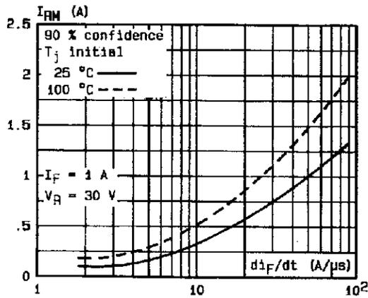
Figure 9. Dynamic parameters versus junction temperature.
