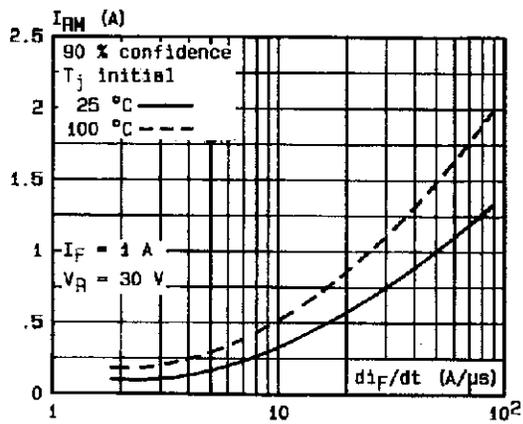
Figure 9. Dynamic parameters versus junction temperature.
